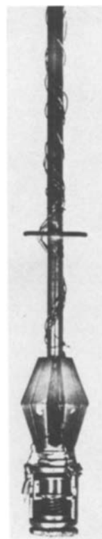
Figure 1 Sample holder for 4 to 300 K ultrasonic measurements.
